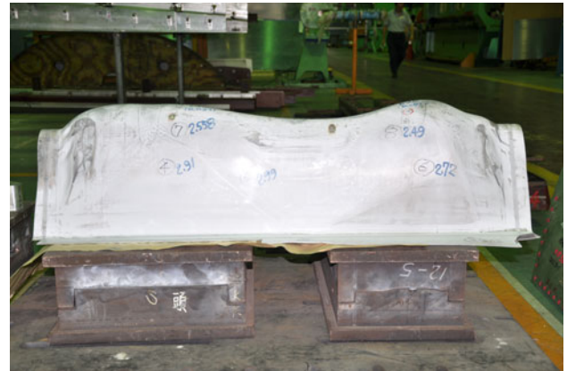
Fig. 10 A gas-formed trough using commercial AA5182, which is far from completion as compared with its counterpart of SP5083
