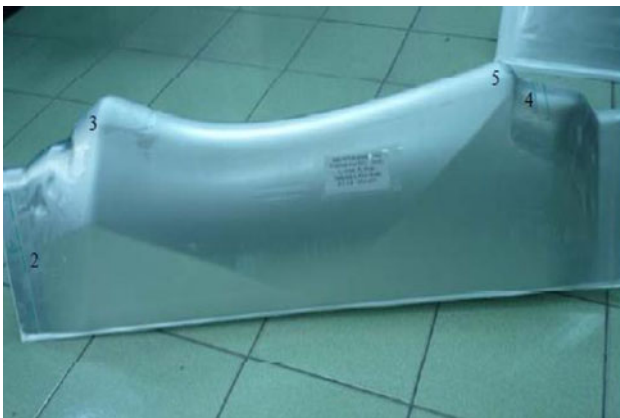
Fig. 5 The trough bears a contour resembling a camel-back with twin humps, formed at 500 °C by gas pressure in ~46 min
